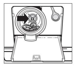
■ Remove any foreign objects (e.g. buttons, coins, etc) and fluff. Turn the impeller by hand to check that it is free to rotate. Any foreign object causing an obstruction should be removed.
